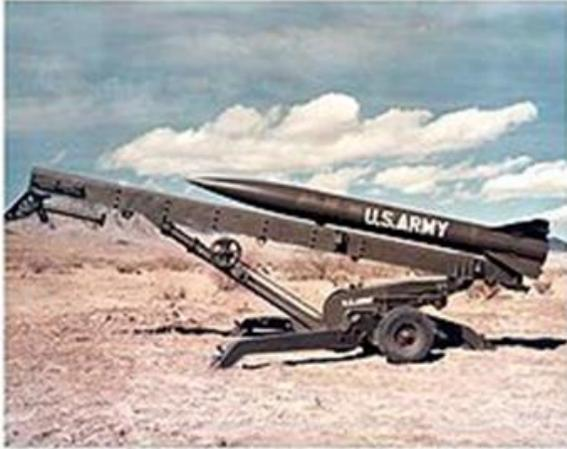
American [MGR-3 Little John](#) missile, measuring 4.4. meters long with a diameter of 32 cm and a weight of 350 kg. Capable of firing a [W45](#) warhead (10 kiloton yield) a distance of 19 km
