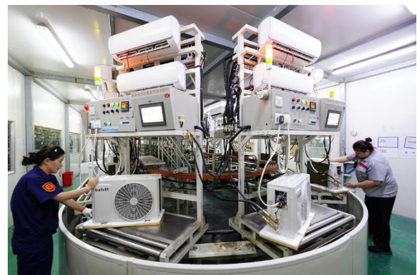
Employees conduct quality inspections on air conditioners using an automated testing system at an air-conditioner manufacturing facility in Fuyang, Anhui Province, China, June 4, 2026. /CFP
